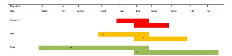
The overlap at mid flow is the region where the two flow control devices have same flow for both inputs and are able to produce mixtures close to 1:1 partial pressure ratio. For 2Mix it is possible to increase the overlapping mid-range if and when necessary.
