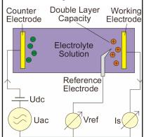
A polarization voltage Udc, superimposed by a small ac voltage Udc is applied to the sample. The response current Is\* and the voltage Vref\* across the electrochemical double layer capacity are measured by amplitude and phase and thus the double layer impedance Z\*=Vref\* / Is\* is determined. In potentiostat or galvanostat mode, Udc is continuously adjusted in order to keep the dc part of Vref or Is at a defined, i.e., constant level.
