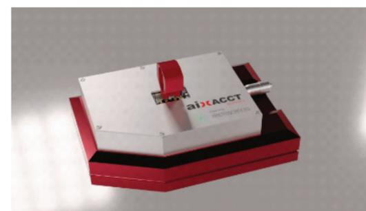
The ESPY31 enables quick and precise measurement of the piezoelectric  $d_{31}$  and  $d_{32}$  coefficients of piezoelectric polymer films or other soft piezoelectric materials such as fibres or membranes. It contains an integrated force measurement cell. It is a highly sensitive measuring device that can also be used to measure other electric properties, like P-E hysteresis or capacitance.
