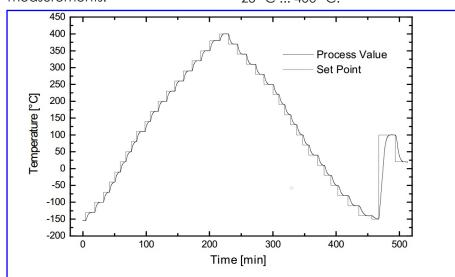
Stabilization characteristics of the sample temperature (process value) compared to temperature set point (step function). Set point step after sample temperature stabilization to 0.1°C accuracy.
